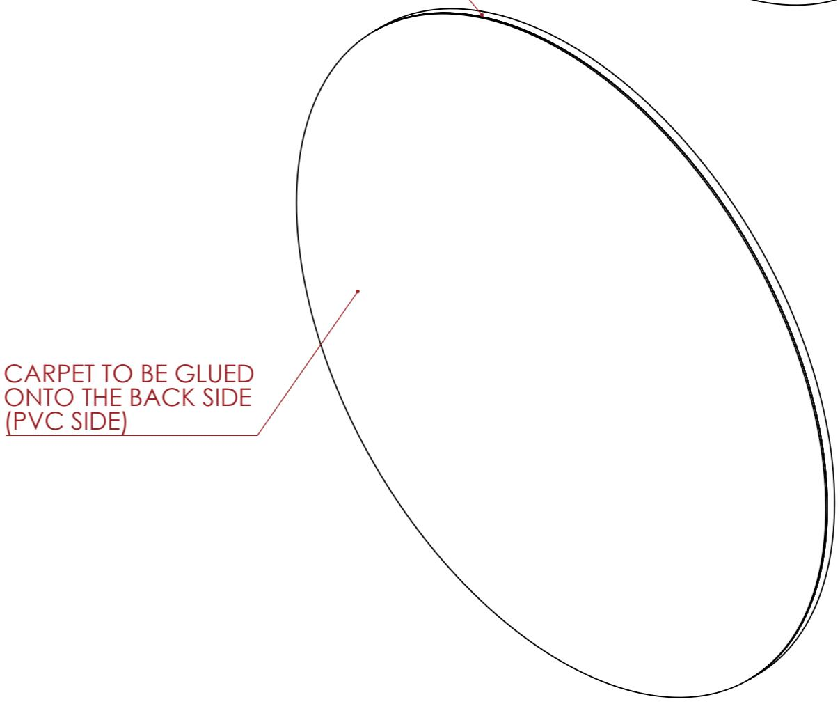
EDGES OF PLYWOOD TO BE ROUNDED FOR EASIER HANDLING
